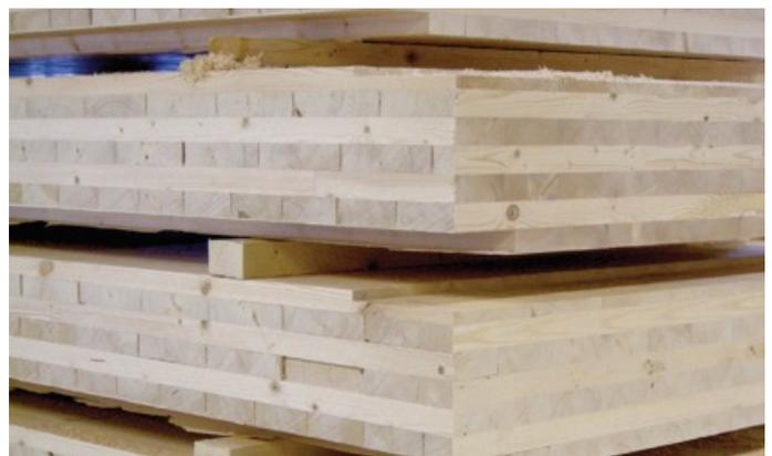
**Figure 1:** Stacked CLT Panels [6]
