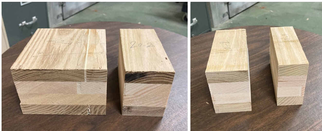
Figure 3. Representatives of DCLT Sample Cut to Random Sizes
