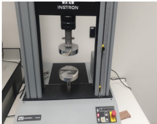
Figure 3. Universal Testing Machine (UTS) with stiff plates
